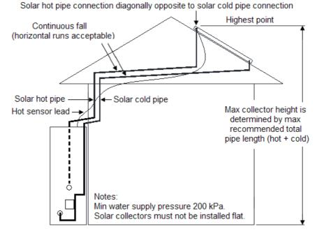
**Solar Pipe Work & Insulation**
