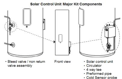
The solar control unit is mounted on the side of the solar storage cylinder and controls system operation. The solar control unit has a power cord which connects to a 240 volt general purpose outlet (refer to 'Installation – Electrical & Electrical Connections' on page 29).
