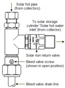
Note: This assembly is to be insulated by plumber
