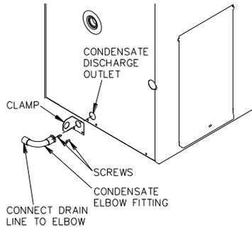
A drain line is recommended to be connected to the condensate elbow to carry the discharge clear of the water heater. The drain line can be extended using 16 mm rigid conduit. The pipe work from the discharge outlet to the drain should be as short as possible and fall all the way from the water heater with no restrictions.
