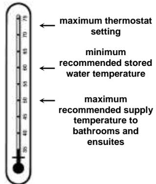
**Note:** AS 3498 requires that a water heater provides the means to inhibit the growth of Legionella bacteria in potable water. This water heater can satisfy this AS 3498 requirement provided it is operating and the thermostat setting is 60°C or higher, including when it is used as an in-series booster water heater for a solar water heater.
