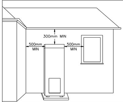
**Note:** \* If these horizontal distances cannot be achieved, AS/NZS 5601.1 states an equivalent horizontal distance measured diagonally from the nearest discharge point of the flue terminal to the opening may be deemed to comply. Check with the local regulator.
