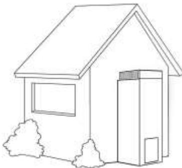
The water heater is to be installed at ground or floor level on a stable fireproof base as acceptable to local authorities. The water heater must also stand vertically upright with the back of the water heater **against or within 25 mm of an external wall** or alternatively against a fireproof screen extending at least 500 mm above, below and either side the flue terminal. Failure to observe this precaution can cause problems in high wind areas.
