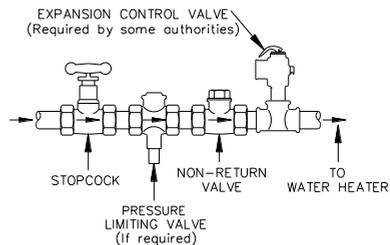
A disconnection union must always be provided at the cold water inlet and hot water outlet on the water heater to allow for disconnection of the water heater.
