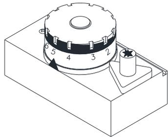
To increase the water temperature to 66°C or 73°C, turn the gas control knob anticlockwise to a setting of '6' or '7' respectively. Refer to [“Hotter Water Increases the Risk of Scald Injury”](#) on page 5.
